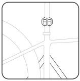
Put some assembly paste on the inside of the seat tube. A brush for this works great. Insert the seatpost. Clamp the frame in a service stand on the seatpost. Give yourself plenty of room to work and walk around the bike.
