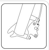
Attach the brakes and shifters to the handlebar. Also bolt the brake calipers to the frame and fork.
