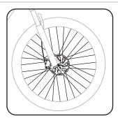
Install the brake rotors on the wheels, and insert the wheels into the frame and fork. Make sure the wheels are properly aligned and does not touch the frame (also quickly check spokes by hand to make sure tension is even) and the tires are in the correct directional orientation.
